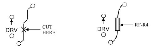
Solder resistor RF-R4 (5.6 k) on the bottom of the board between the two pads located at either end of the cut trace segment. Use the minimum lead length necessary. Position the resistor so that its leads do not touch any adjacent pads or traces. Solder the resistor on the bottom of the board.
