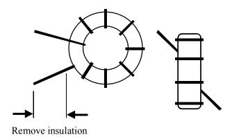
Spread out the turns of L1 so they occupy about 80-90% of the core's circumference.
